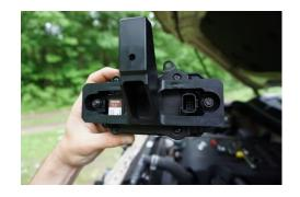
Step 4: Mount current assembly to truck using (1) screw, (1) lock nut, (2) washers. Re-connect wiring harness. Cable tie wiring harness to drivers side horn bracket and clip as shown.
