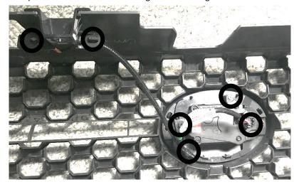
**Step 3:**Assemble TSS Sensor and 10052 Bracket and Cover using (2) screws, (2) lock nuts, (4) washers.
